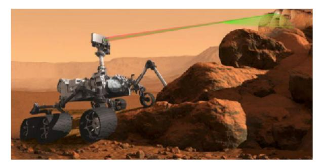
This artist's illustration shows how NASA's Mars 2020 rover will use Supercam, a laser instrument that can provide imaging, chemical composition analysis, and mineralogy.
