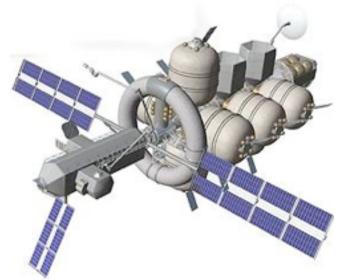
NASA concept Study for a Non-Atmospheric Universal Transport Intended for Lengthy US space eXploration, Nautilus-X shows several inflatable modules and a rotating torus providing artificial gravity. The dream vehicle could make round-trips to many solar system destinations <a href="http://www.space-travel.com/reports/A Reusable Manned">http://www.space-travel.com/reports/A Reusable Manned</a>
