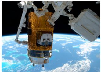
JAXA robotic Cargo ship at ISS
