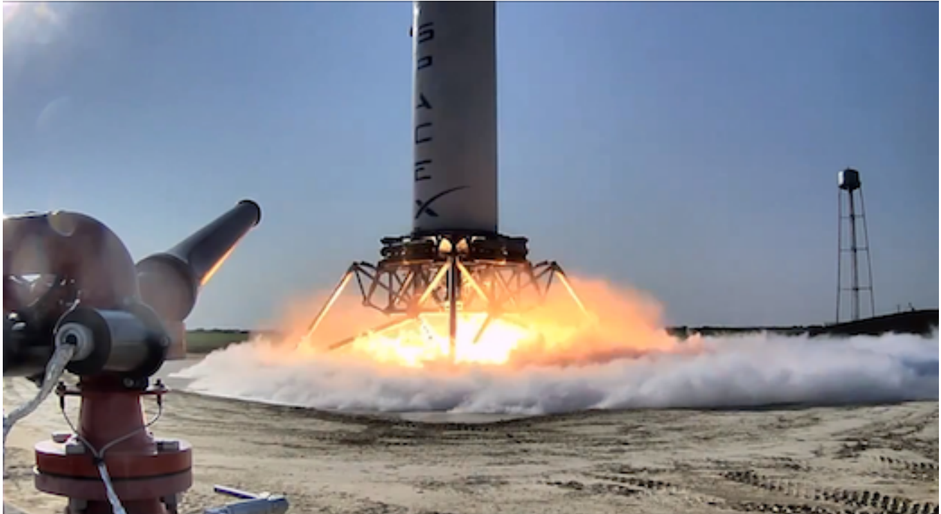
Space-X tests its “Grasshopper” – A demonstrator of a vertical takeoff, vertical landing “reusable” rocket
