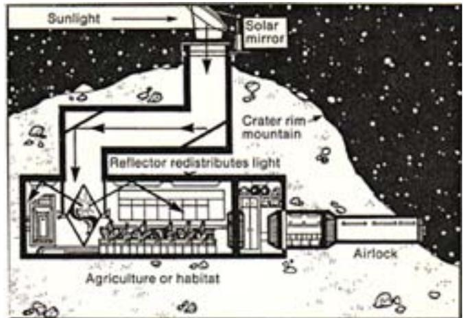
**UNDERGROUND POLAR HABITAT:** Sunlight piped in from heliostat. L. Ortiz/NASA. As drawn, this would work if the Moon's axial tilt were zero. In fact it is 1.5° and to be able to catch the sun's rays at all times of the month, the heliostat would have to be on a tower at least 2,000 ft. above all surrounding terrain. If the habitat were not at the exact pole, the tower would have to be even higher. So much for a nice idea.
