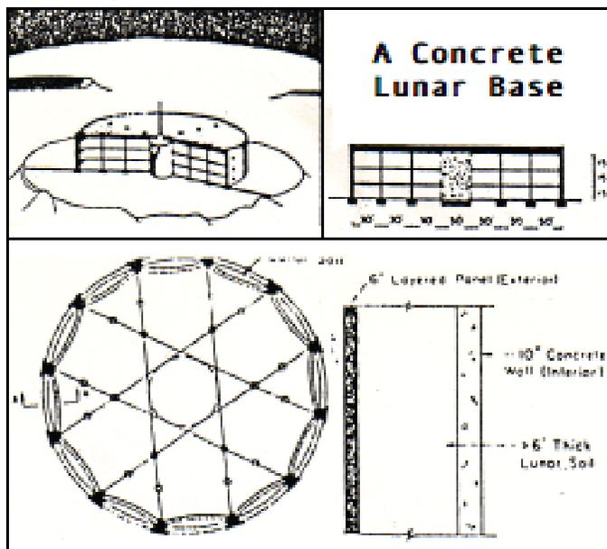
So instead of taking to the Moon a collection of Earth-made modules to assemble into a prefab ready-to-do-nothing outpost, with good intentions of someday working towards some early industrial projects, Lin's group would start with lunar industry, enough of it to process cement, his steel cables and panel connectors, his concrete wall, floor and roof panels, etc. The outpost itself would be the first project
