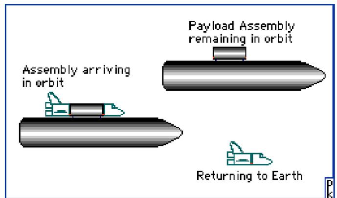
In the radically reinvented space transportation system, the return "orbiter-tug" is much smaller than today's shuttle (smaller wings & tail and no payload bay. All these weight savings are reinvested in a larger payload structure that remains attached to the External Tank which is taken all the way to orbit, for minimal extra fuel.
